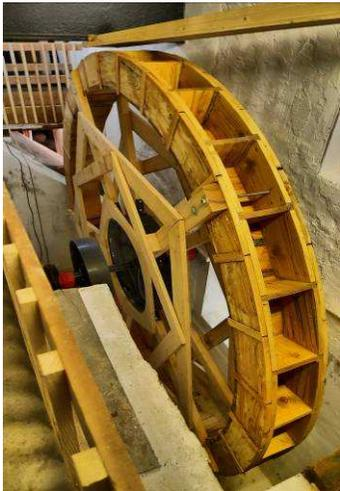
Water powered paddle wheel, in 1865 four of these were in use as well as 5 sets of grindstones
